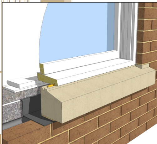
Typical installation detail
